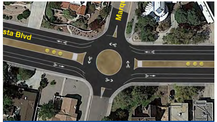
Full Median with Roundabout
