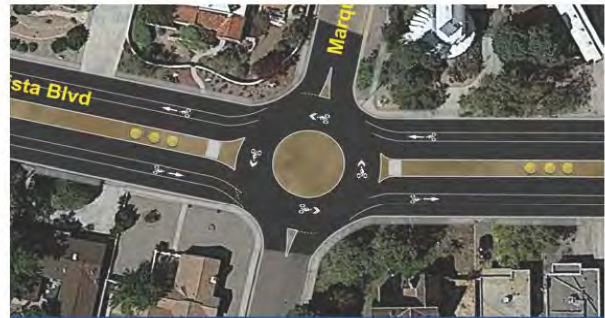
Full Median with Roundabout
