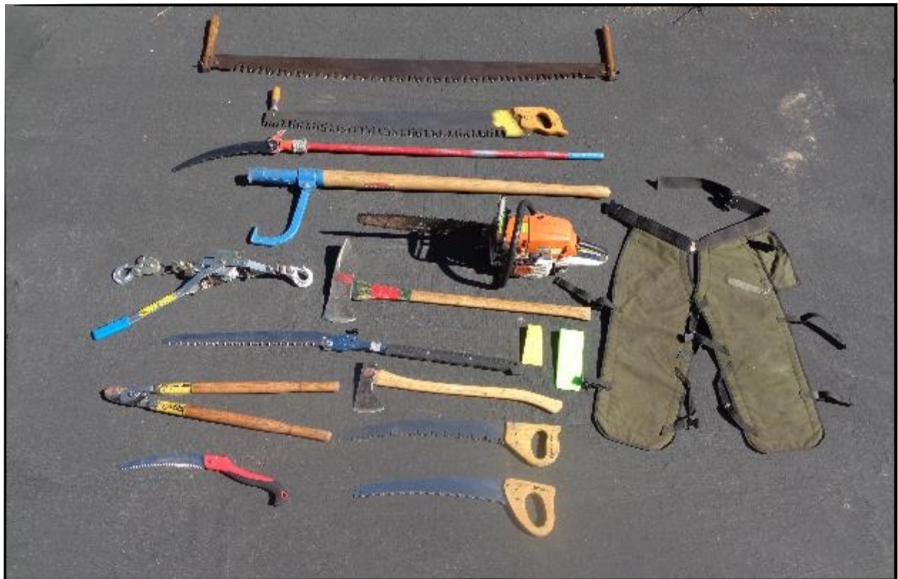
Tool names starting in the lower left corner – short Corona folding pruning saw, 18-inch Corona pruning saw, 21-inch Corona pruning saw, long-handle loppers, Collins Hudson Bay axe, 19-inch Katanaboy folding saw, bucking wedge, felling wedge, chain saw protective leg chaps, hoist, Pulaski, chain saw, cant hook, pole saw, one-person crosscut saw, two-person crosscut saw.
