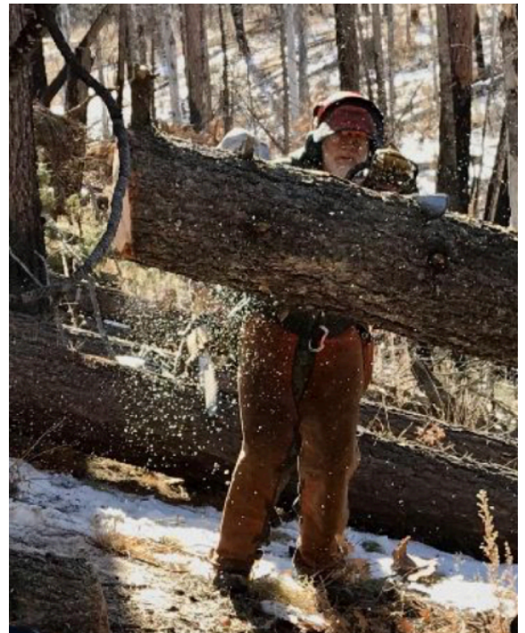
Sam cutting a large log with a Stihl MS-261 saw with an 18-inch bar
