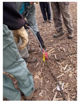
Attaching the griphoist's wire rope to the chain with a closeable hook. Again, each part of the system, including connecting pieces, needs to be rated for the anticipated load.
