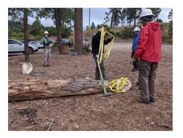
This log will work for practice. The padded straps can be wrapped around the anchor tree in the background. Every link in the system needs to be rated for (at least) the weight of the object being moved.
