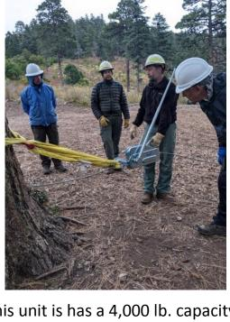
This unit is has a 4,000 lb. capacity, and the smaller one is rated for 2,000 lbs. That's still a ton! Note the telescoping handle for ease of use.
