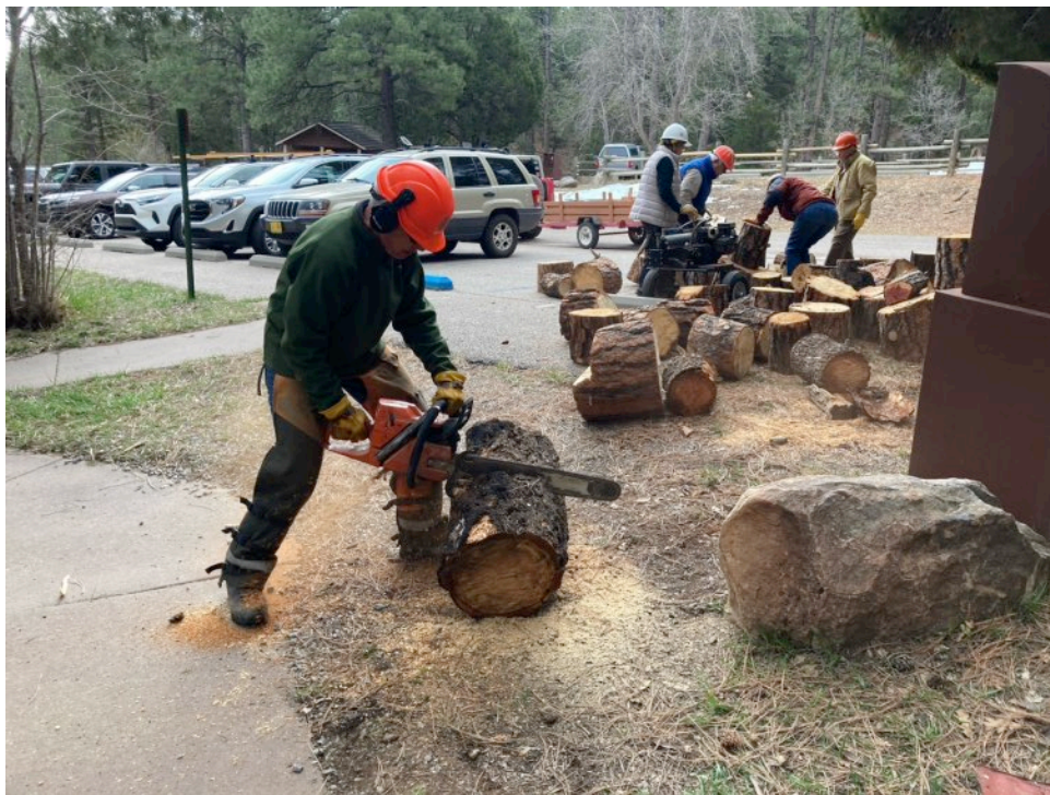
Steve uses a chainsaw to buck a log into shorter rounds before splitting.
