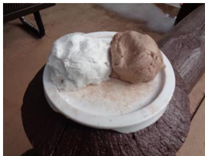
White resin and brown hardener are mixed manually
